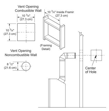
Figure 9 - Vent Opening Requirements
